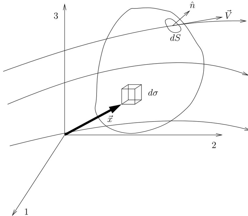
FIGURE 5.14. An arbitrary control volume chosen in some fluid flow. An elemental area on the controls surface  $dS$  and an elemental volume  $d\sigma$  within the control volume are also shown. Note that in most coordinate systems we may not be able to indicate a position vector  $\vec{x}$ .
