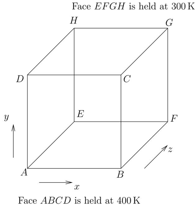
FIGURE 6.6. A unit cube. The governing equation is given by equation (6.1.25). The front and the rear faces are held at 400 K and 300 K respectively. The rest of the faces are adiabatic
