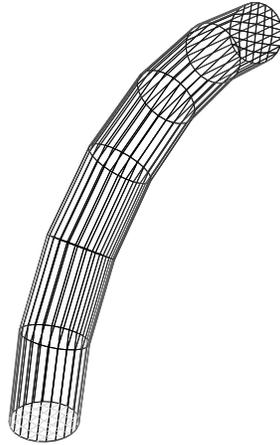
FIGURE 6.35. A  $7 \times 7$  elliptic grid generated in a unit circle in the  $xy$  plane is scaled and stacked in the  $\theta$ -direction to generate a three-dimensional grid in a torus. A quarter of the torus is shown. There are seven grid planes along the  $\theta$ -axis. Only grids on the inlet, exit, and boundaries are shown for clarity
