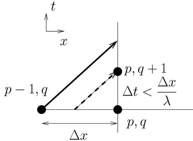
FIGURE 3.35. graphical representation of characteristics on a mesh where  $\sigma < 1$  for FTBS. The solid arrow points to the zone of influence from the grid point  $p - 1, q$ . The dashed arrow points from the the zone of dependence of the grid point  $p, q + 1$ . The grid point  $p, q + 1$  is in the zone of influence of the interval  $[x_{p-1}, x_p]$
