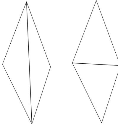
FIGURE 6.23. Two Possible Triangulations with the Four Nodes
