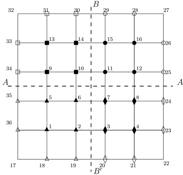
FIGURE A.2. Grid points used to solve Laplace's equation on a unit square at the origin in the first quadrant. The domain is shown divided into four parts using two broken lines:  $A - A'$ ,  $B - B'$ . The grid points are indicated appropriately. It should be noted that to compute some of these grid points data from adjacent domains is required. This data needs to be made available as and when required.
