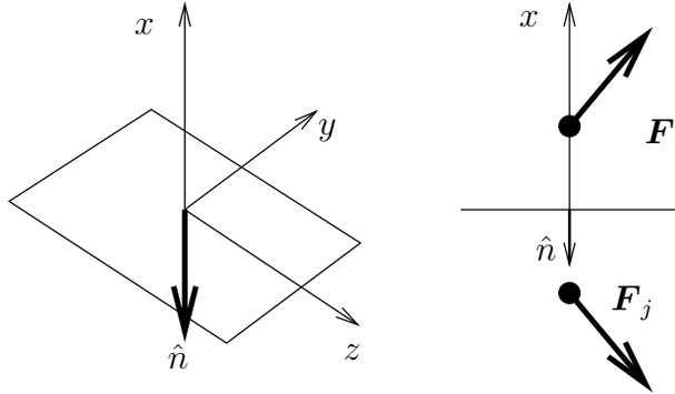
FIGURE 6.3. A surface element, a unit vector  $\hat{n}$  normal to that element and pointed out of the cell, and points on either side of the element are shown. A “local” coordinate system is also indicated. If the element represents a solid wall, the mass flux through the surface element is zero
