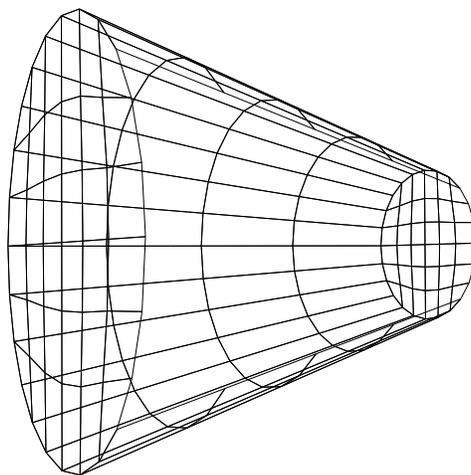
FIGURE 6.34. A  $7 \times 7$  elliptic grid generated in a unit circle in the  $xy$  plane is scaled and stacked in the  $z$ -direction to generate a three-dimensional grid in a converging conical nozzle. There are five grid planes along the  $z$ -axis. Only grids on the inlet, exit, bottom, top, and back faces are shown for clarity
