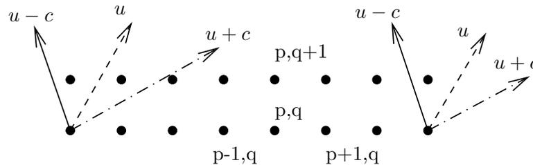
FIGURE 4.7. Characteristics at a subsonic inlet and a subsonic exit at time level  $q$ . Grid points at time level  $q + 1$  are also shown.
