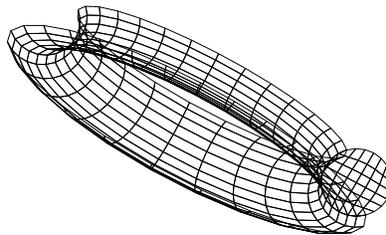
FIGURE 6.36. A  $7 \times 7$  elliptic grid generated in a unit circle in the  $xy$  plane is stacked along a circle to generate a three dimensional grid in a full torus. The  $7 \times 7$  grid is shown. Grids are also shown on the bottom and back faces for clarity.
