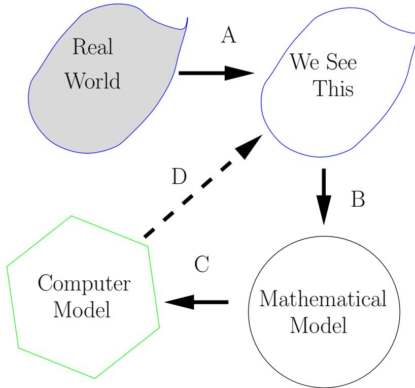
FIGURE 8.1. How CFD works. The polygon at the end is our approximation to the circle. The process marked “A” is perception. The process marked “B” maybe abstraction. The process “C” is the CFD. Finally the process marked “D” would be validation
