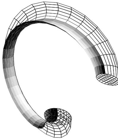
FIGURE 6.33. A  $7 \times 7$  elliptic grid generated in a unit circle in the  $xy$  plane is scaled and stacked along the helix  $(0.2t, 0.1 \cos t, 0.1 \sin t)$  to generate a three-dimensional grid in a helical tube. There are twenty eight grid planes stacked along the helix. Only grids on the inlet, exit, bottom, and side coordinate surfaces are shown for clarity
