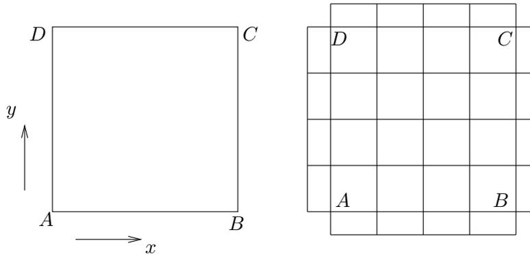
FIGURE 6.5. A unit square. The governing equation is given by equation (6.1.25).  $AB$  is held at 400 K and  $CD$  is held at 300 K. The  $BC$  and  $AD$  are adiabatic. A  $4 \times 4$  cell discretisation is shown. Note the pseudo volumes indicated on the sides
