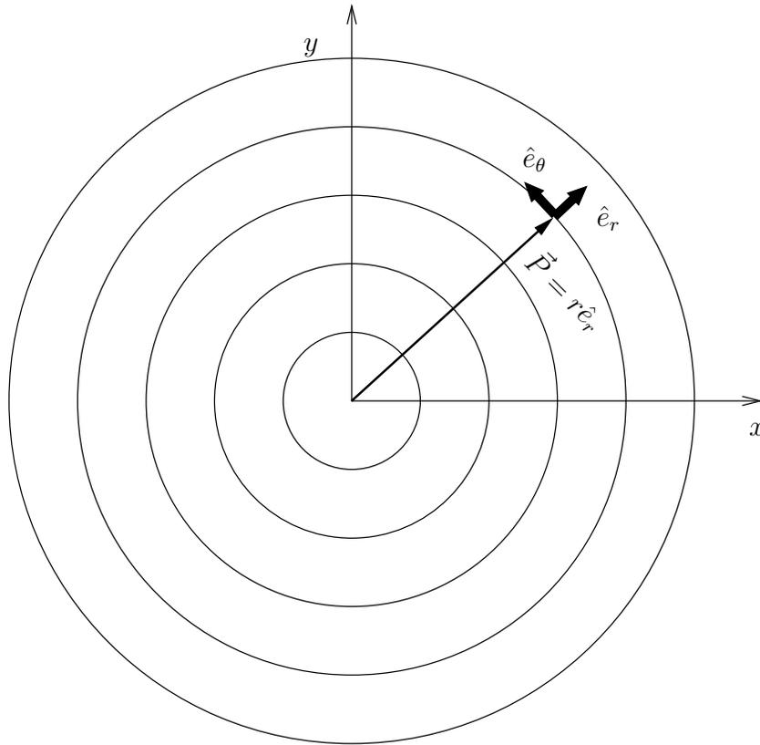
FIGURE 5.8. The position vector in polar coordinates is given by  $\vec{P} = r\hat{e}_r$ . At first glance it seems as though there is no  $\theta$  dependence. However  $\hat{e}_r$  is a function of  $\theta$  as is  $\hat{e}_\theta$ . Only the constant  $r$  coordinate lines are shown.
