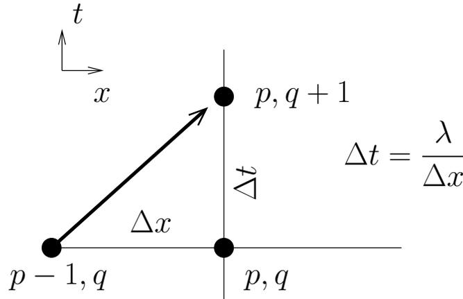
FIGURE 3.34. Yet another way to look at stability, FTBS has the upstream influence. The arrow indicates flow of information ( $u$ ). This figure represents the case of  $\sigma = 1$ . The arrow, in fact, is a characteristic. Since  $\sigma = 1$ , the zone of influence and the zone of dependence happen to be grid points
