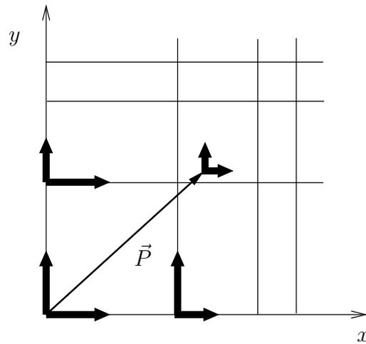
FIGURE 5.9. A “log-log” coordinate system. We have a rectangular coordinate system, however the unit vectors are still a function of position making it impossible to write the position vector drawn  $\vec{P}$  as a linear combination of the basis vectors.
