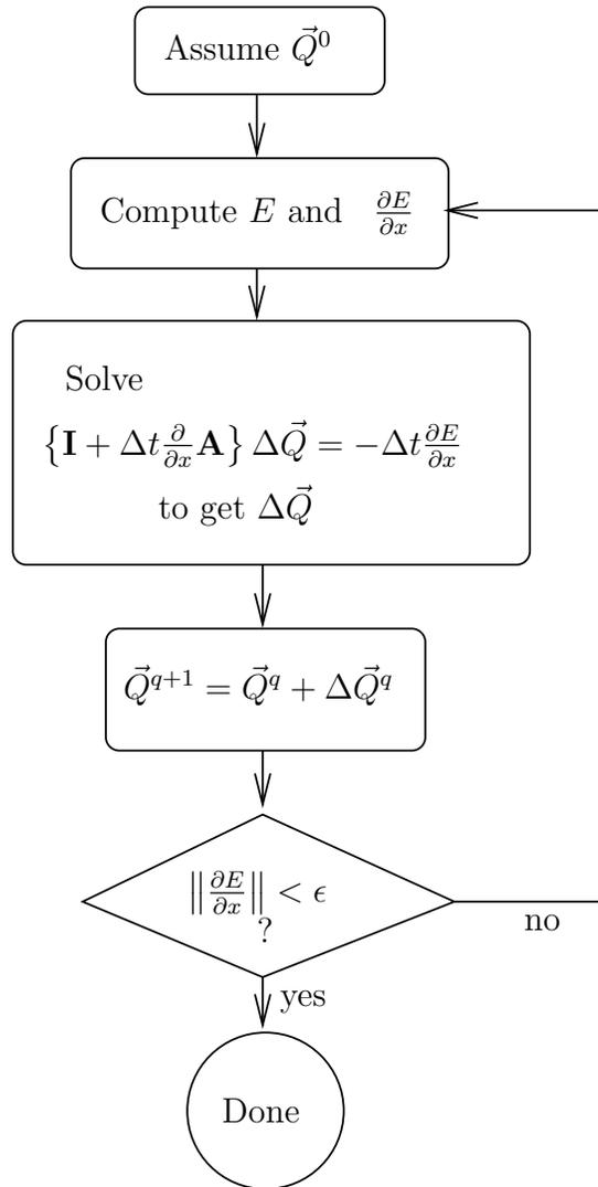
FIGURE 4.8. Algorithm for solving one-dimensional Euler equation
