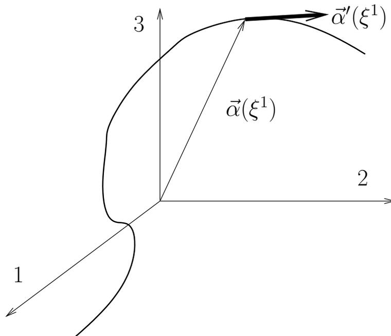
FIGURE 5.10. A coordinate line belonging to a three dimensional generalised coordinate system. This line is shown embedded in our usual Cartesian coordinate system.  $\vec{\alpha}$  is shown as a function of  $\xi^1$  alone as the other two,  $\xi^2$  and  $\xi^3$  are held constant to obtain this line. The local tangent vector is one of the basis vectors for the generalised coordinates
