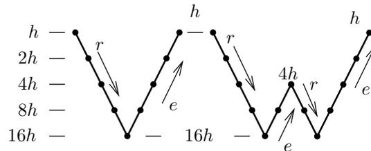
FIGURE 7.9. The V-cycle and the W-cycle.  $r$ , the residue, is passed down a left limb from a fine grid to a coarse grid and  $e$ , the correction, is passed up the right limb from a coarse grid to a fine grid.  $h, 2h, 4h, 8h,$  and  $16h$ , indicate the grid size at the dots at the corresponding level on the limbs
