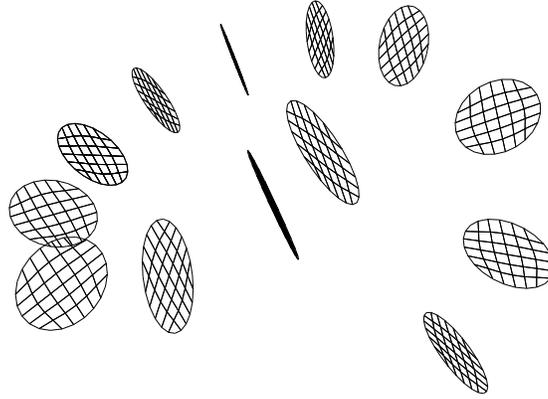
FIGURE 6.32. A  $7 \times 7$  elliptic grid generated in a unit circle in the  $xy$  plane is scaled and stacked along the helix  $(0.2t, 0.1 \cos t, 0.1 \sin t)$  to generate a three-dimensional grid in a helical tube. There are twenty eight grid planes stacked along the helix
