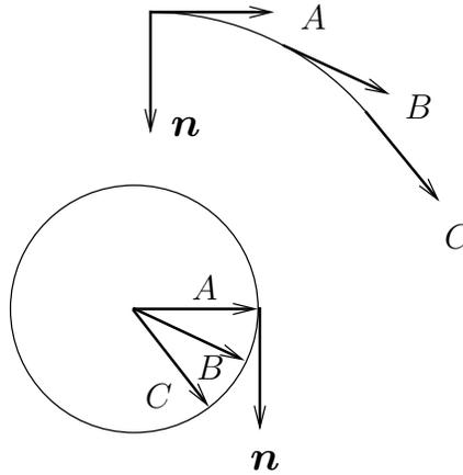
FIGURE 6.13. A planar curve is shown with tangents at three different points. These tangent vectors are shown located at a single point. The arrow heads lie on a unit circle since the tangent vectors in this case are unit vectors
