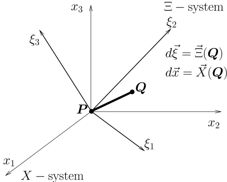
FIGURE 5.11. Figure 5.5 is redrawn and zoomed. The origin of our Cartesian coordinate system is translated to the point  $P$ . The differential element  $PQ$  is now represented in terms of the translated coordinate system and a similar system of the generalised coordinates.
