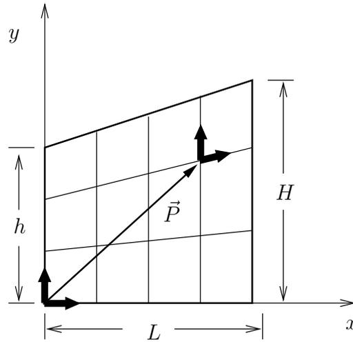
FIGURE 5.7. The basis vectors at the origin and the basis vectors at some other point are clearly not the same. The position vector,  $\vec{P}$  is geometrically very easy to draw. It cannot be written simply as a linear combination of some basis vector in the coordinate system shown here.
