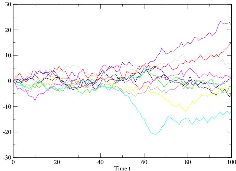
FIGURE 7.8. Ten paths with  $\mu = 0$  and  $\sigma = 1$  obtained by integrating equation (7.2.5) over a hundred time steps using the explicit Euler's scheme and a  $\Delta t = 1$
