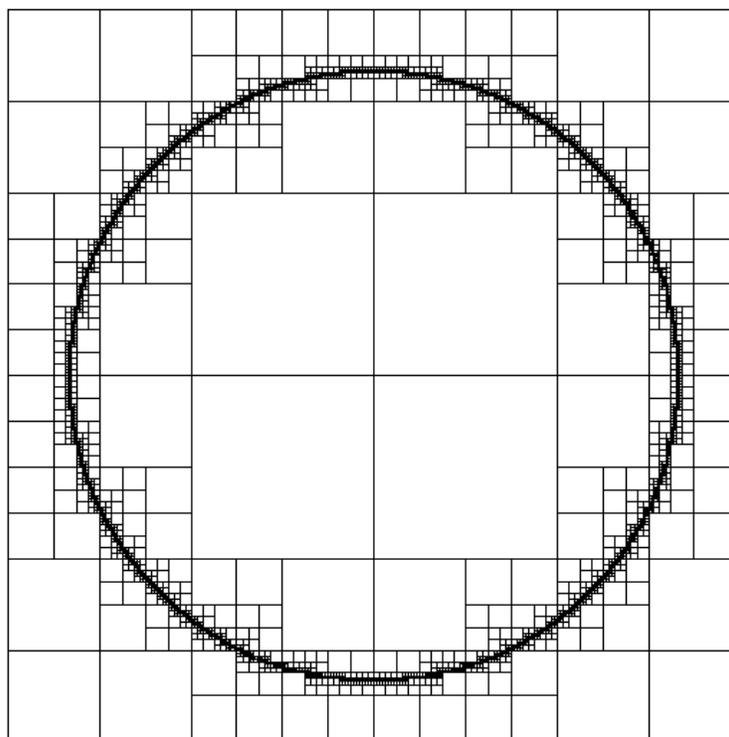
FIGURE 6.29. An unstructured Cartesian mesh generated to capture the circle  $x^2 + y^2 = 1$ , the mesh goes down ten levels
