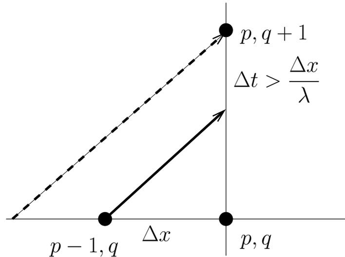
FIGURE 3.36. graphical representation of characteristics on a mesh where  $\sigma > 1$  for FTBS. The solid arrow points to the zone of influence from the grid point  $p-1, q$ . The dashed arrow points from the zone of dependence of the grid point  $p, q+1$ . The grid point  $p, q+1$  is outside the zone of influence of the interval  $[x_{p-1}, x_p]$
