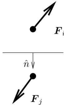
FIGURE 6.4.  $F_i$  and  $F_j$  are mass fluxes in the interior and pseudo cells.  $\hat{n}$  is a unit normal pointing out of the domain. For a viscous flow, not only is the mass flux through the surface element zero, the velocity at the boundary is zero
