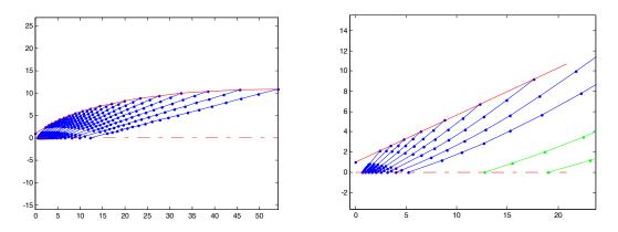
Example of plot of characteristic fabric calculated for (a) nozzle design, (b) straight line nozzle flow. For clarity I have omitted the negative characteristics from the plots. But they can also be plotted.
