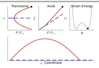
**Example**: A pinned-pinned beam undergoing axial loading.
