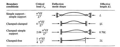
Effective lengths of beams with different boundary conditions (Figure from Brush and Almroth 1975)
