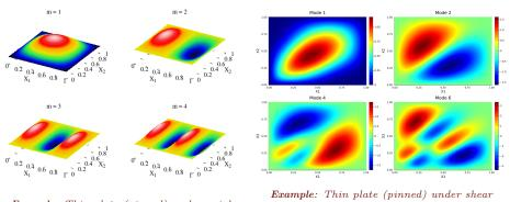
Example: Thin plate (pinned) under axial loading
