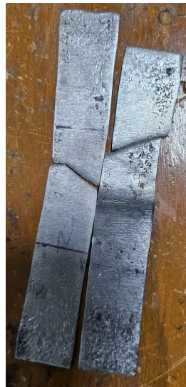
Failed mild steel specimens (under uni-axial tension) ◀ ◻ ▶
