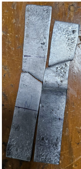
Failed mild steel specimens (under uni-axial tension)
