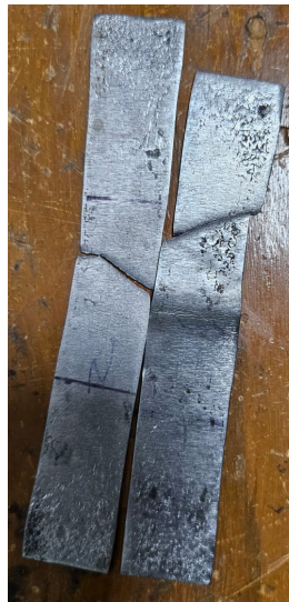
Failed mild steel specimens (under uni-axial tension) ◀ ◻ ▶
