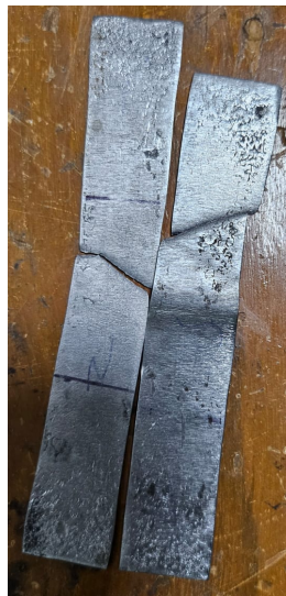
Failed mild steel specimens (under uni-axial tension)
