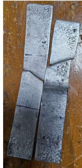
Failed mild steel specimens (under uni-axial tension) ◀ ◻ ▶
