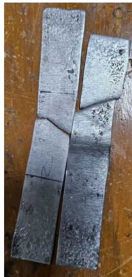
Failed mild steel specimens (under uni-axial tension)
