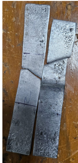
Failed mild steel specimens (under uni-axial tension) ◀ ◻ ▶
