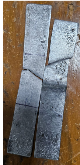
Failed mild steel specimens (under uni-axial tension)
