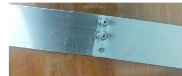
Bearing hole elongation — 0.5 mm plate
