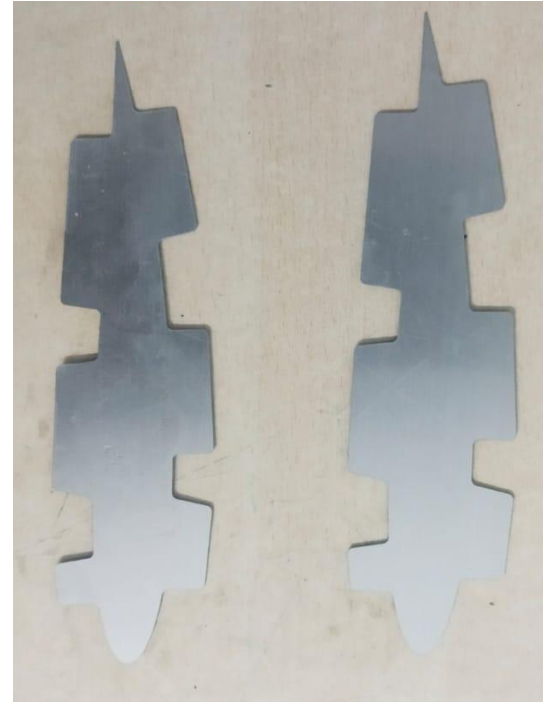
Design 1 - Fabricated Rib Before Bending
