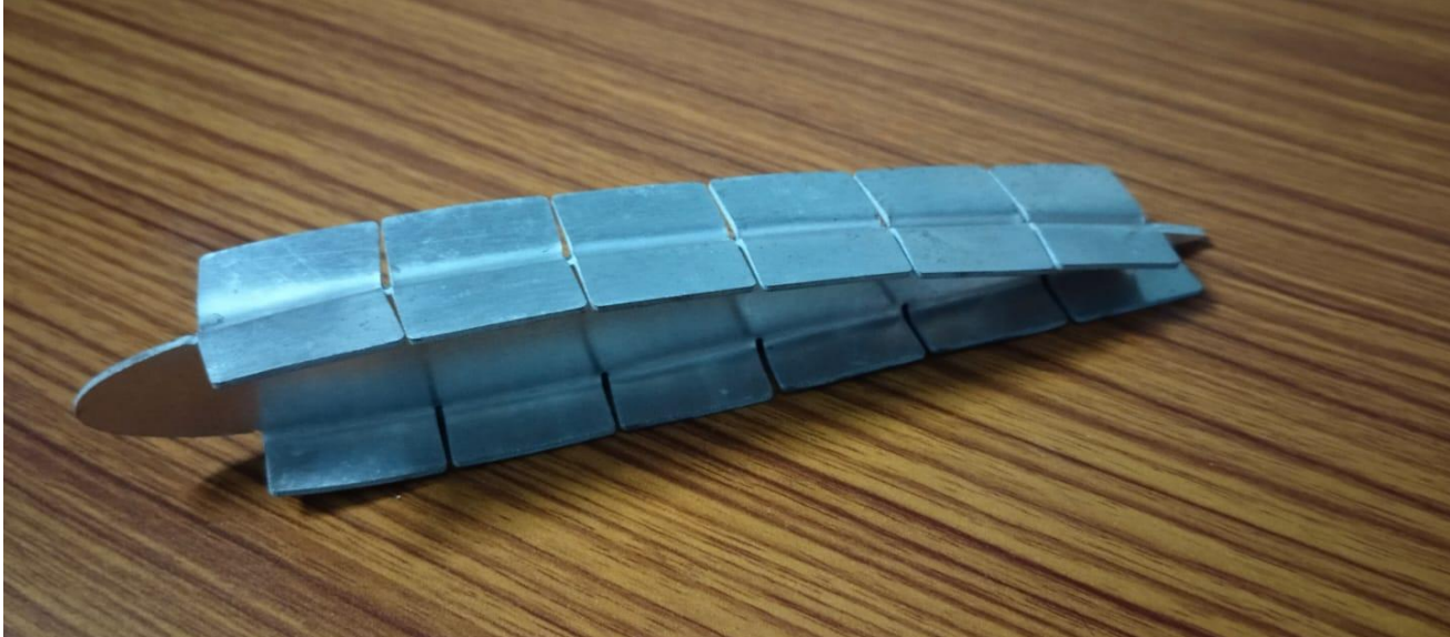
Design 3 - Fabricated Rib After Bending
