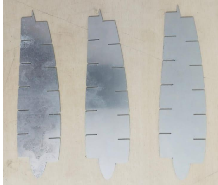
Design 3 - Fabricated Rib Before Bending
