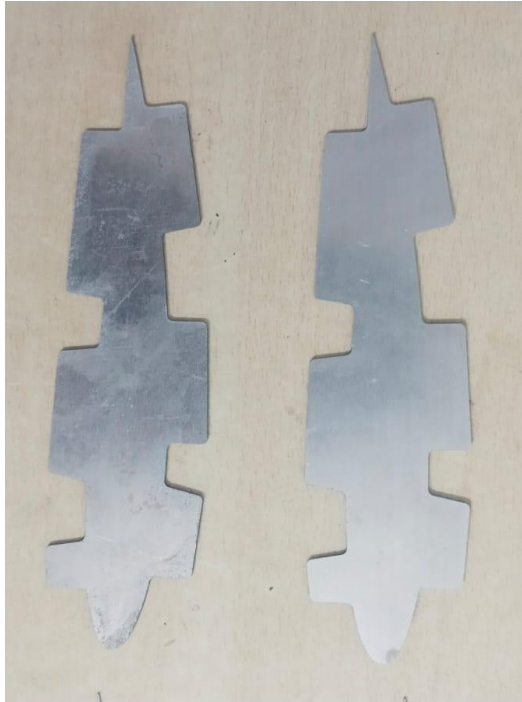
Design 1 - Fabricated Rib Before Bending
