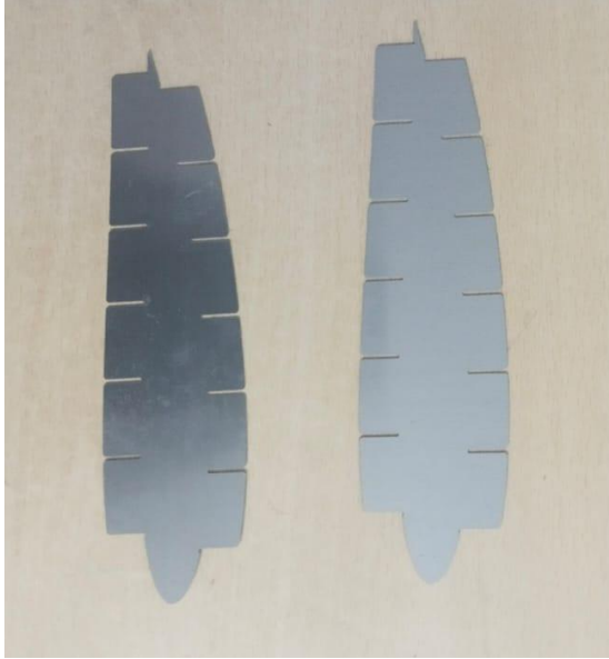
Design 3 - Fabricated Rib Before Bending
