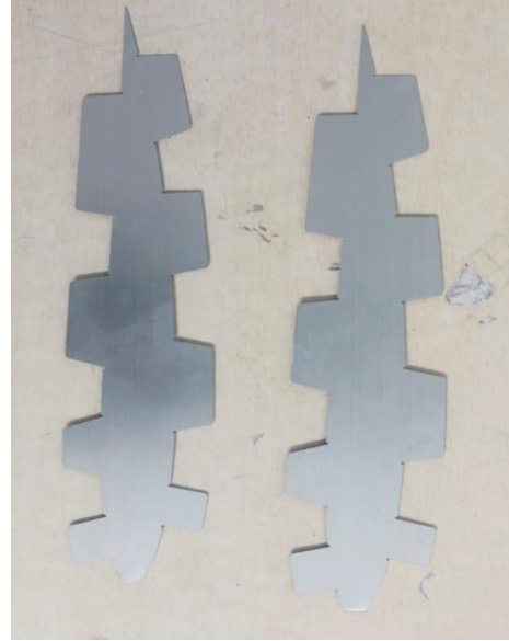
Design 2 - Fabricated Rib Before Bending
