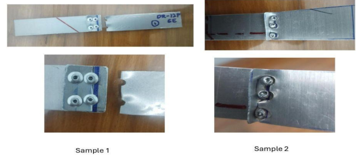
Fig. 6.1 — Tearing failure curves & specimen photos (Week 3)
