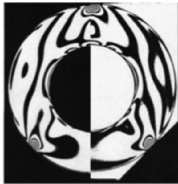
Fig. 3.12 Isochromatics on a black and bright background of an annular disc loaded at three points
