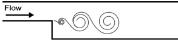
Figure 1.6: A schematic representation of periodic vortex shedding in dump combustor. Often this periodic shedding couples to system acoustics causing generation of thermoacoustic oscillations in the system.
